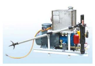
YYTZ26-1B unit: about 300 kg weight, with explosion-proof motor, power consumption about 8 degrees per hour.
